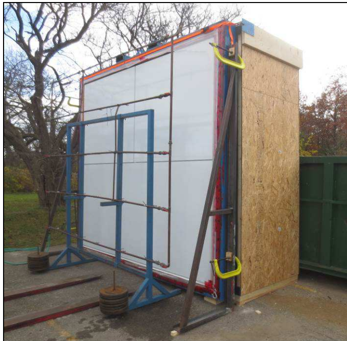
Figure C2 - Spray rack Set up for water penetration
