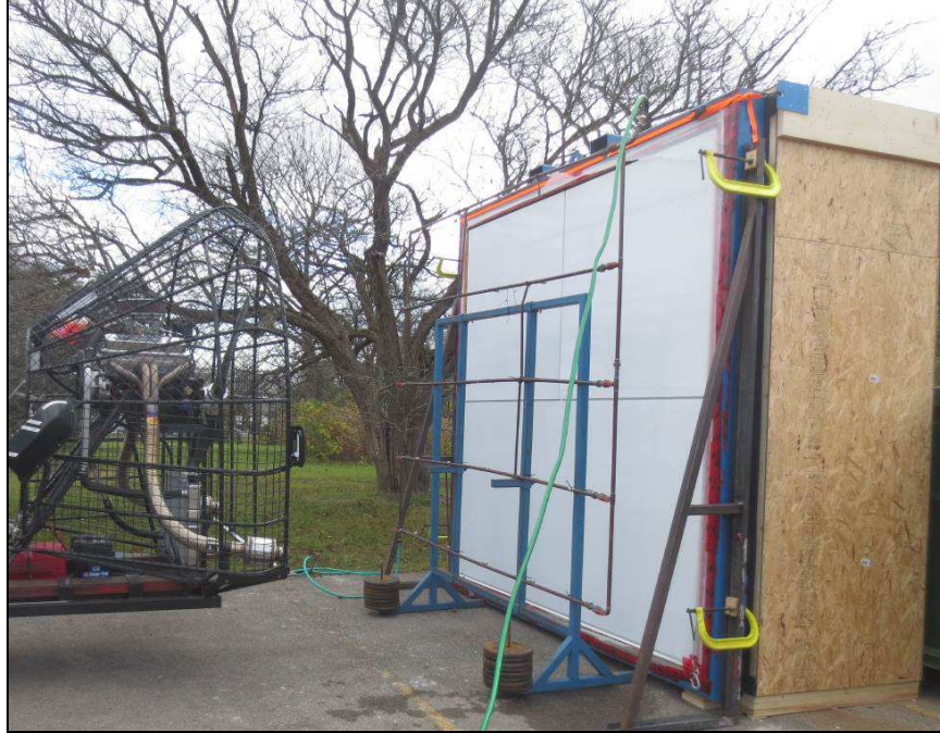
Figure C3 - Wind Machine setup to simulate Dynamic Pressure (AAMA 501.1-05)
